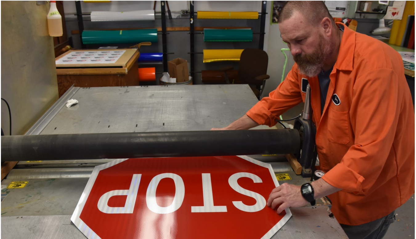
Jerry Sommers is one of two fabricators inside the five-man Sullivan County Sign Shop, which calls the Barryville depot home. Here he works on rolling a vinyl stop sign onto its reflective backing, ensuring wind and weather don't tear it apart.
