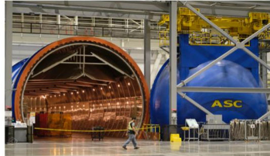
A worker walks past a giant autoclave, which provides superheated pressure needed in the construction of the new 777X composite wing at the Boeing 777X Composite Wing Center in Everett, Washington. Stephen Brashear/Getty Images
